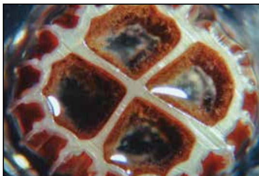
FIGURE 3. Biological growth on the carrier forms a thin biofilm on the media in an MBBR system
