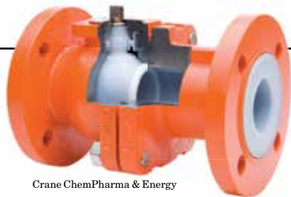
FIGURE 3. The Xomox XLB lined ball valve offers smaller actuators for reduced costs and space and weight savings. It allows installation in space-restricted areas in parallel piping systems and is fully lined with permeation-resistant PFA material as a barrier to corrosion
