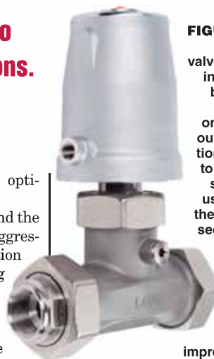
FIGURE 1. The New Generation diaphragm valve provides safety, efficiency and simplicity via a central union nut that offers a non-corrosive connection, homogeneous temperature behavior, an even surface pressure, and a high-pressure rating up to 240 psi (for water use only)
